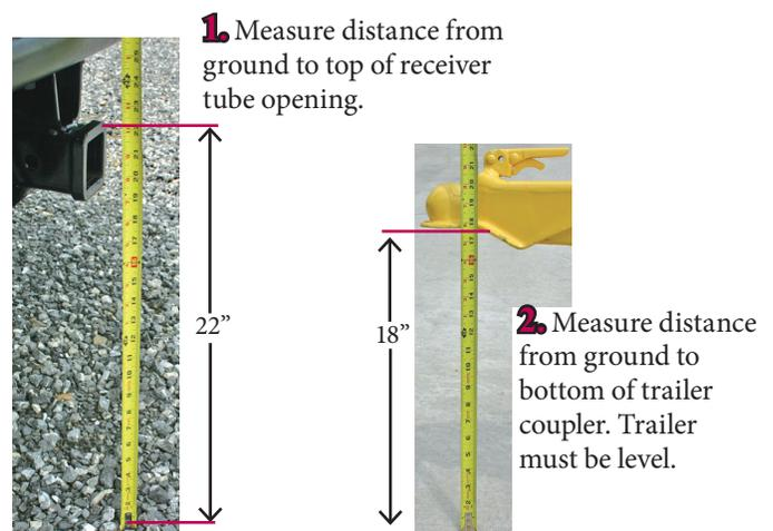
1. Measure distance from ground to top of receiver tube opening.
